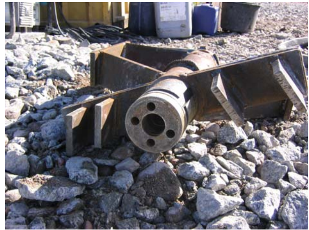
Figure 3 Peripheral conduits for water and central part of hollow stem for binder transport.
